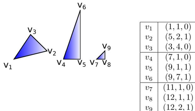
We previously assigned those triangles to a BVH node and now need to determine if that node should be split once more. For that, determine an optimal split plane using the *surface area heuristic* and the sweeping method along the horizontal axis. Determine the costs of every meaningful split and identify the one with the lowest costs. The costs associated with traversing the tree are the same as those associated with intersecting a ray with a triangle.
